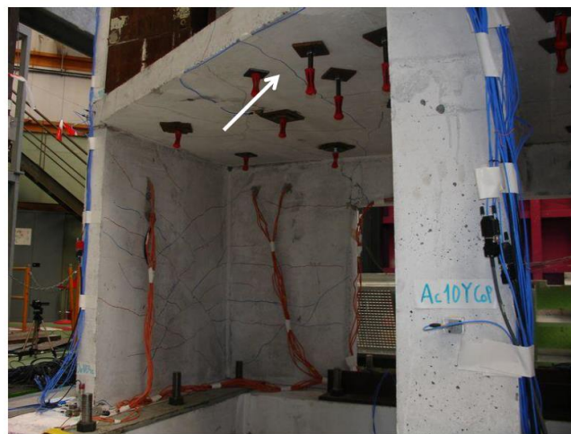
Figure 22: Final state of SMART 2013 (DEN, 2014)
